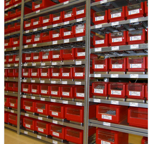
Weight-sensored bins report quantity on hand continuously to SmartStock Select.
