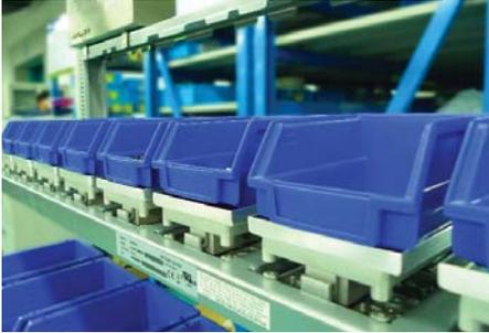
eTurns eVMI solution with a standard rack with sensors sitting under bins
