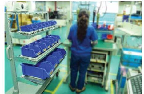
eTurns wireless, battery-operated, mobile carts with eVMI sensors under bins of parts
